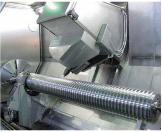
Turning and milling on same setting with highest precision requirements.
