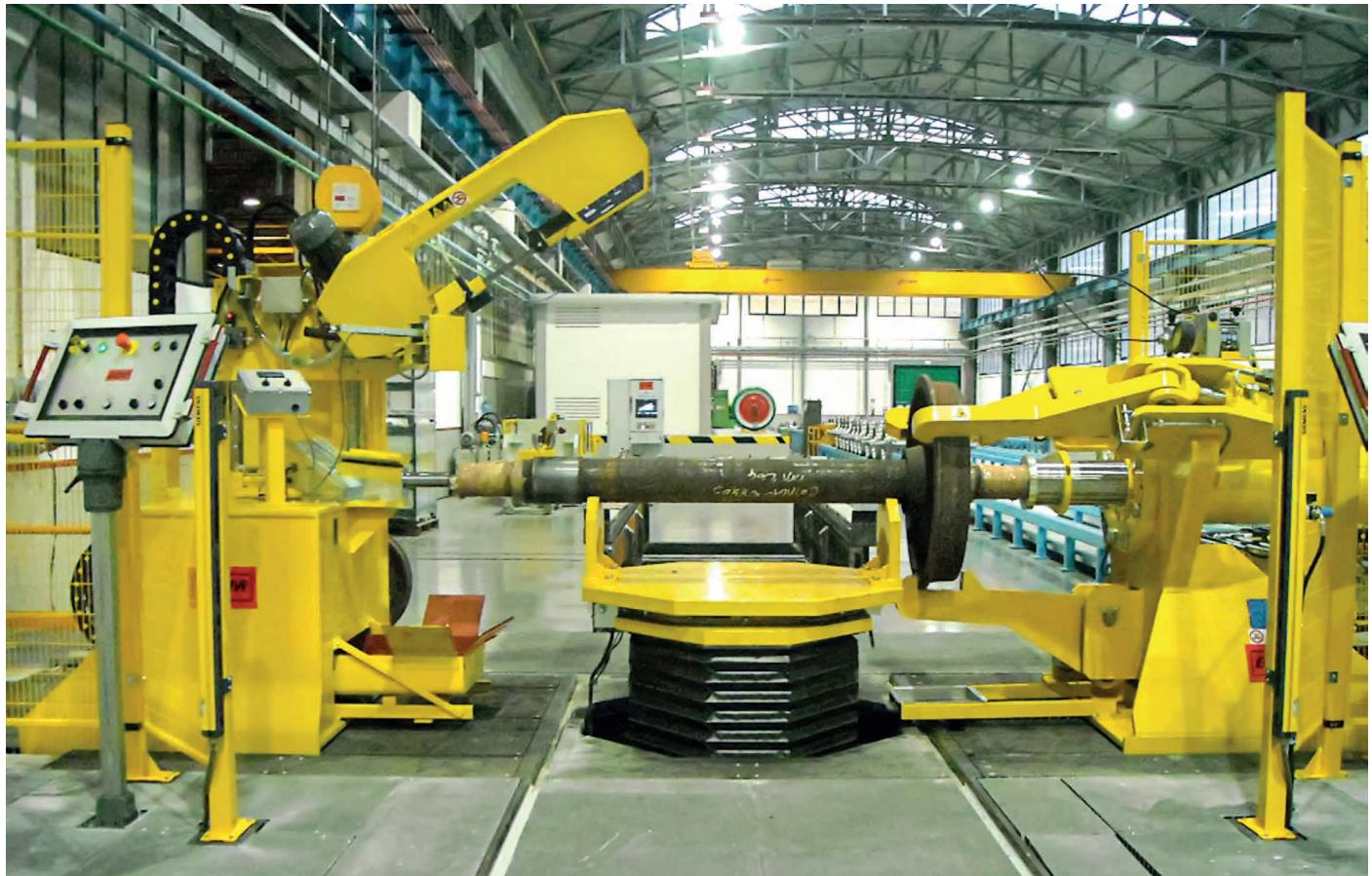
**Machine for Cutting Tyres and Demounting Wheels**
